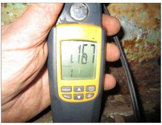
Span 1 Beam 3: (PAR) CORROSION ALONG BOTH FACES OF WEB AND EDGES OF BOTH FLANGES UP TO FULL LENGTH X 10" HIGH DOWN TO 0.16" RESIDUAL WEB, FULL LENGTH X 4" WIDE DOWN TO 0.23" RESIDUAL TOP FLANGE, AND FULL LENGTH X 4" WIDE DOWN TO 0.22" RESIDUAL BOTTOM FLANGE
